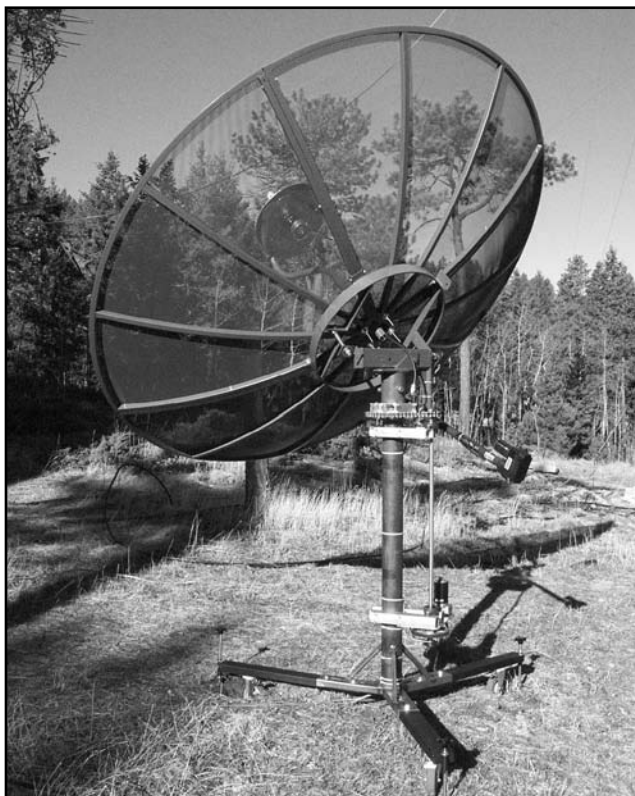
Fig 69—A completed TVRO dish Az-EI mounting system is shown, using a jackscrew elevation drive. (WØLMD photo.)
